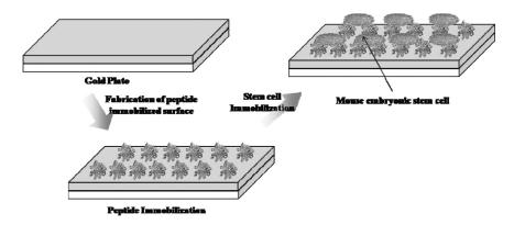
**FIGURE 1** The schematic representation of the cell immobilization on oligopeptide- modified gold substrate.
